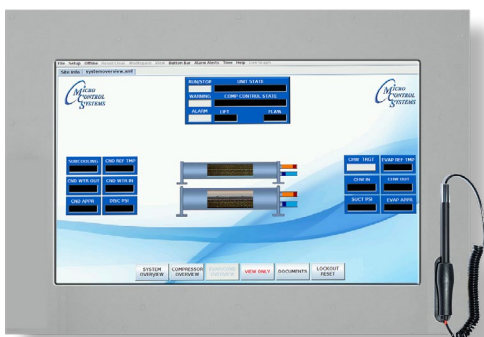
EVAPORATOR CONDENSER OVERVIEW SCREEN
